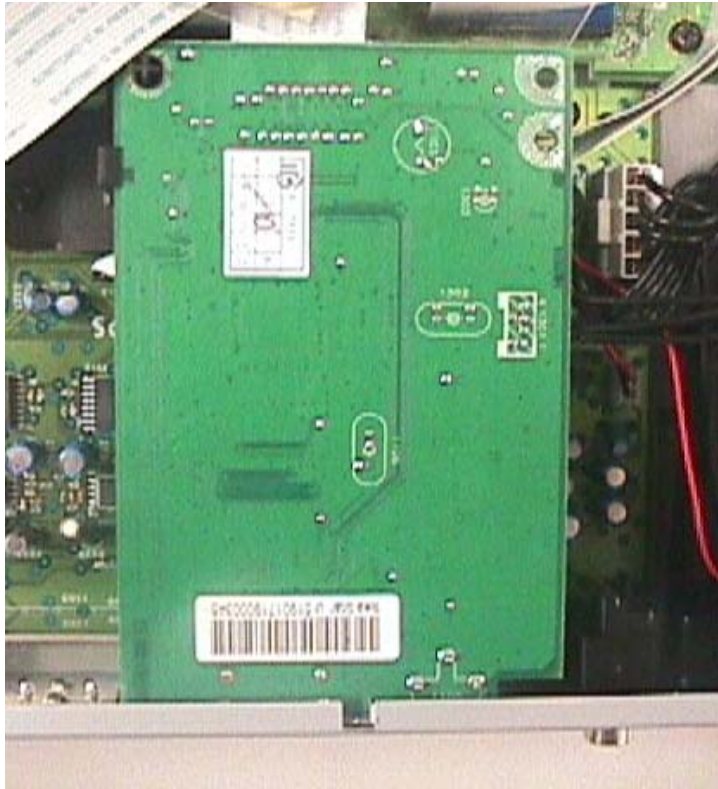
Figure 12 – HDMI Board Service Position (HDMI Shield Removed)
